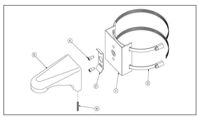
Figure 1. SWM-PA Pole Adapter Locator Drawing
